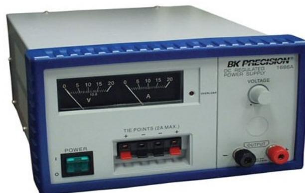
In the model at the right, "tie" points are provided to allow monitoring output voltage with a more
