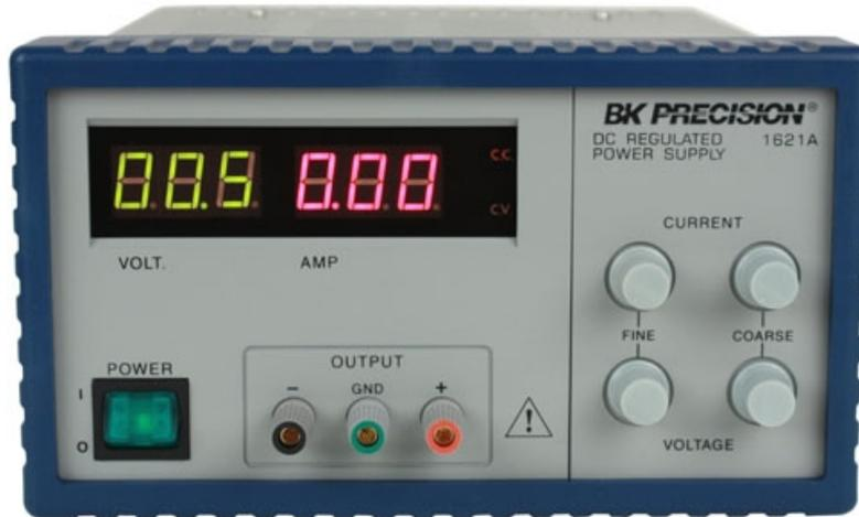
This power supply outputs one adjustable voltage, which is indicated by the one set of banana jack terminals. The above arrangement of output terminals with the ground terminal between the + and - terminals is the most common and makes connecting either terminal to ground using a metal shorting bar very convenient. This is useful when you want one of the terminals to be referenced to ground. Of course, the same thing can be done with a piece of wire or a jumper wire with stackable banana plugs.
